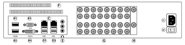
Figure 3: A-Series Hybrid 2UA and F2A System back panel configuration B
