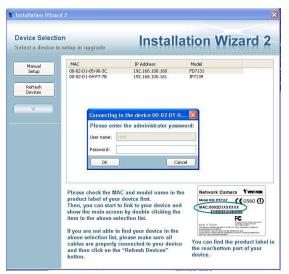
Enter the root password for the Vivotek camera. If you have not set up the camera previously, the default password is blank.
